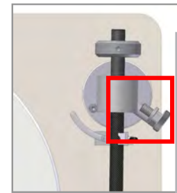
Illustration 3 : Maximum antiskating (Screw is screwed in)
