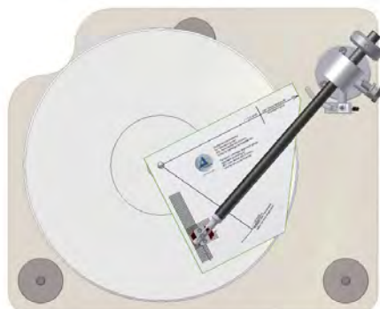
Pic. 10: Alignment of the cartridge
