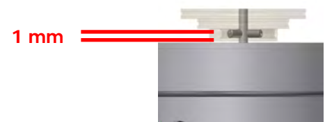
Pic. 12: Mounting the pulley
